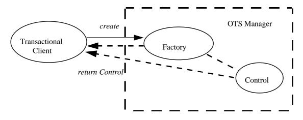
Figure 7. Transaction initialization in OTS.
