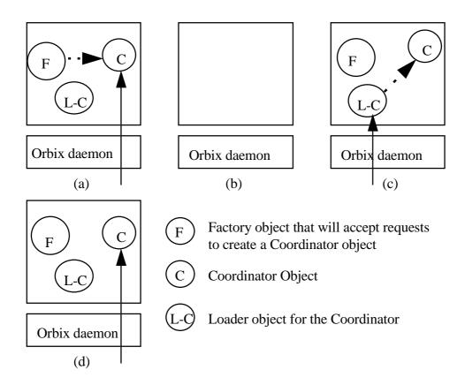
Figure 13. Using Loader Object to Implement the Recovery.
