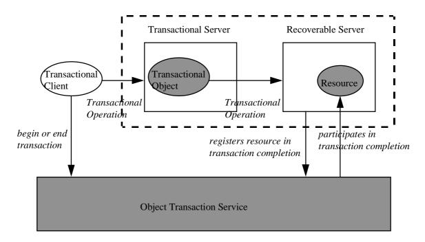
Figure 4. Overview of object transaction service.
