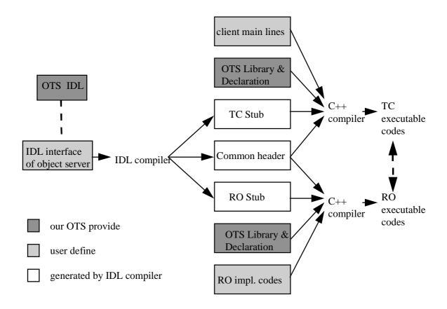
Figure 6. The OTS programming development environment.
