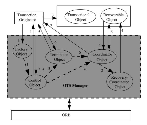
Figure 5. The functional diagram of the applications and the OTS manager.
