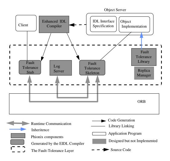
Figure 6. The architecture of the fault tolerance layer in Phoinix.
