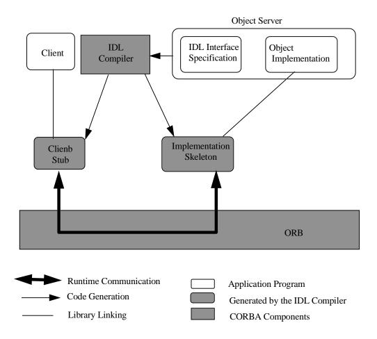
Figure 2. The illustration of Common Object Request Broker Architecture (CORBA).
