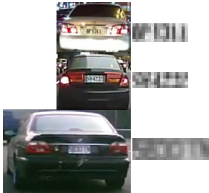
Fig. 10 Three blurred sample license plate images used in the experiments. (From top to bottom) The actual characters of the license plates are 8P-1311, SV-4232 and 5830-TN. (From left to right) Low-resolution vehicle image, and the cropped license plate region.
