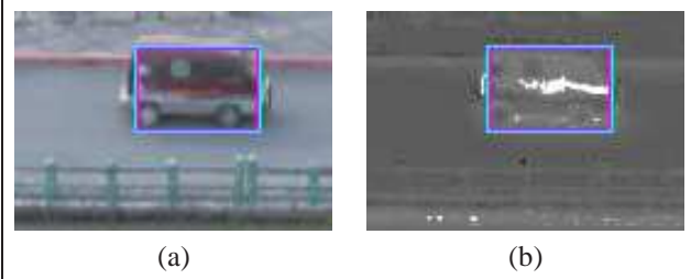
Figure 1. (a) A cropped image frame. (b) The compound likelihood image of (a).
